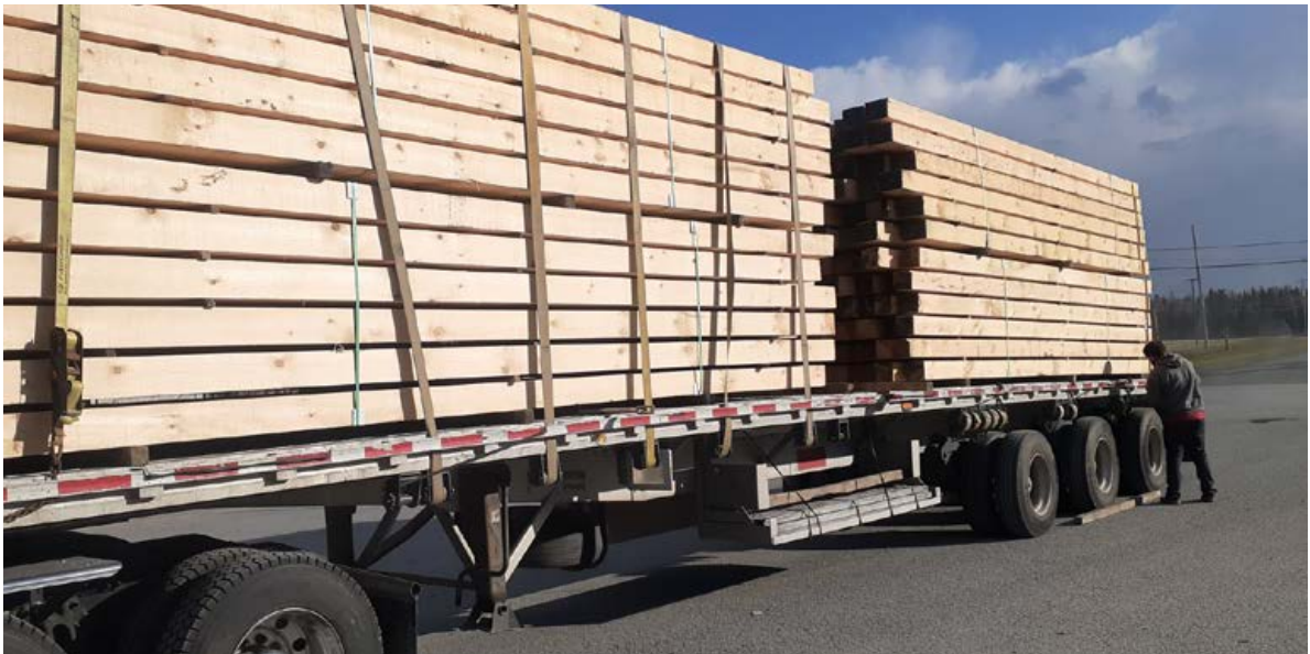
Figure 1 • A Timber Components Shipment Ready for Delivery to a Timber Framer for Fabrication
