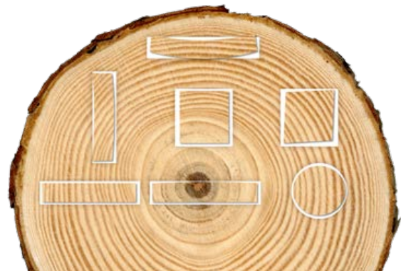
Figure 5 - Dimensional Changes Associated with the Drying of a Green Timber Elements
